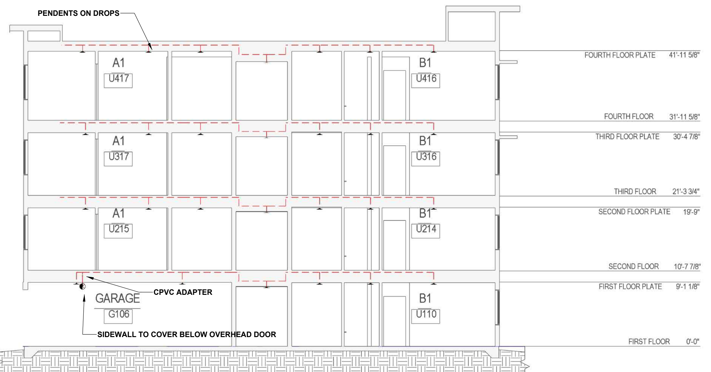
B BUILDING SECTION SCALE: 1/8" = 1'-0"
