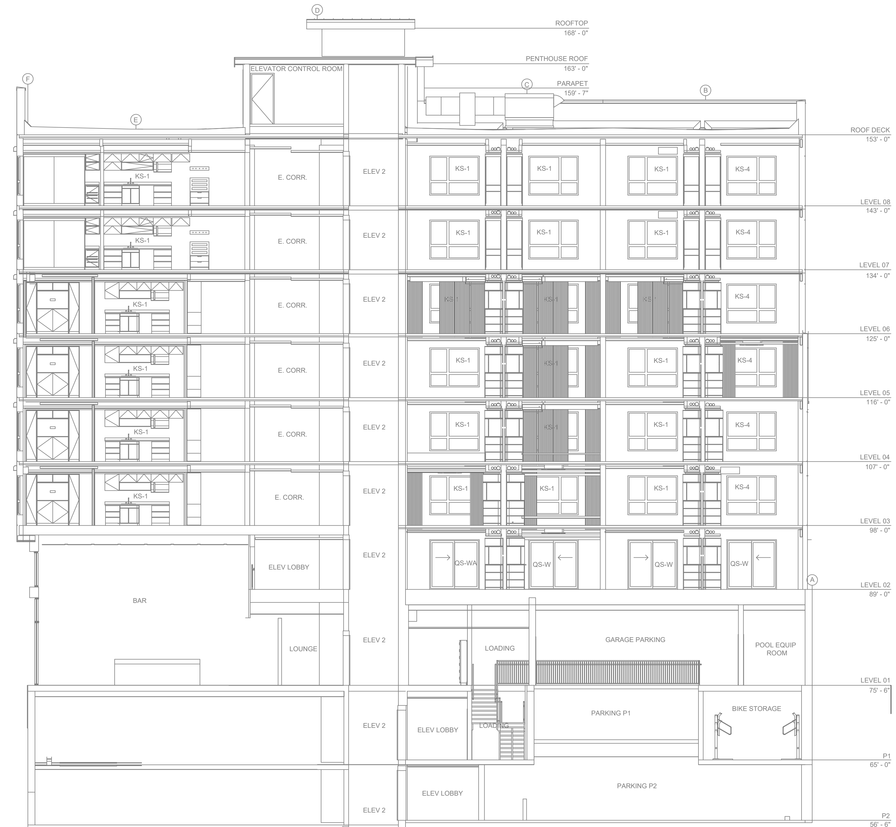
A BUILDING SECTION SCALE: 1/8" = 1'-0"
