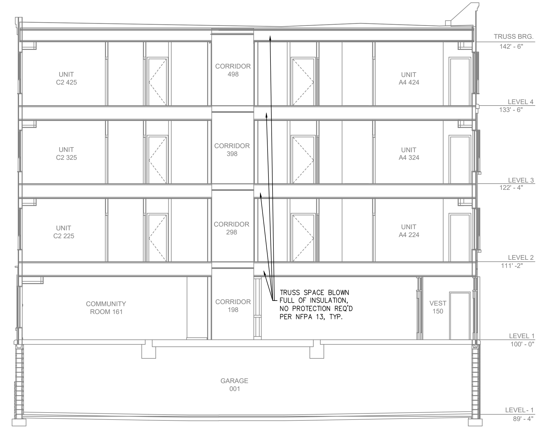
A BUILDING SECTION SCALE = 1/8" : 1'-0"
